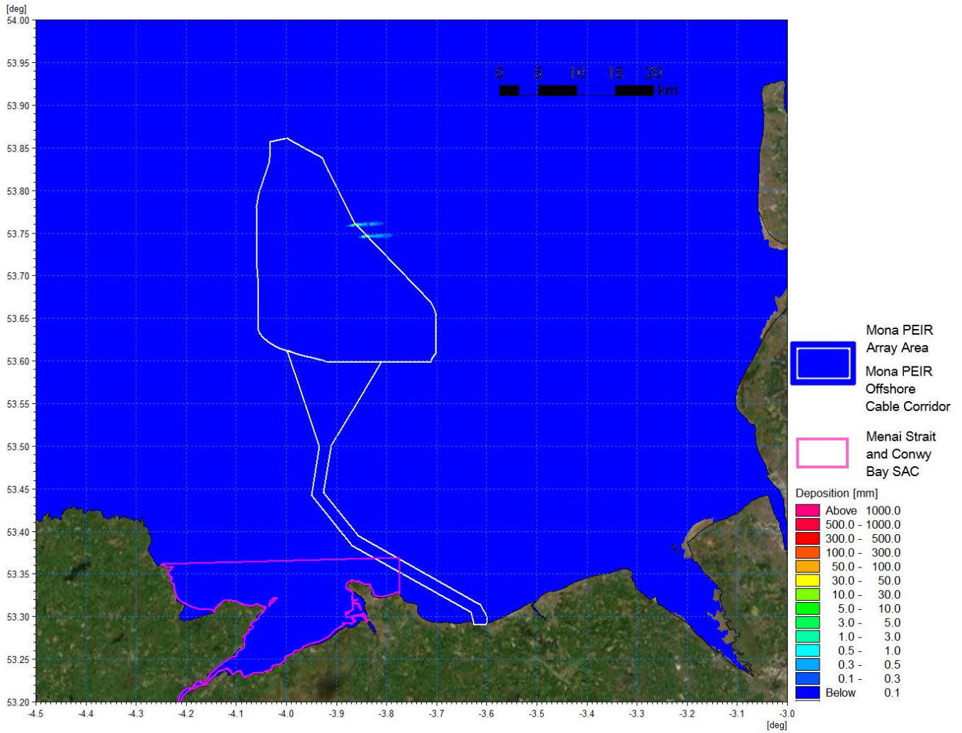
Figure 1.120: Average sedimentation during pile installation – scenario A.
